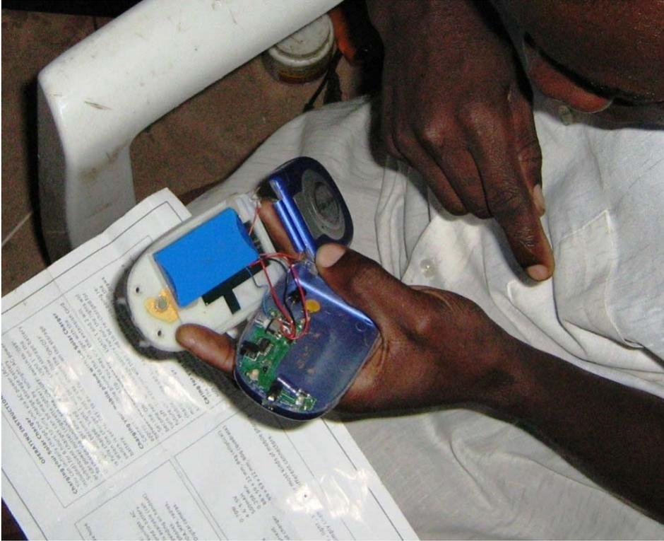
Figure 3b. Solar Charger being repaired in Bungoma town
